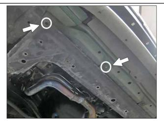
Locate the two holes in the lower radiator support, and remove the bolt in the forward hole. Save this bolt for future use. [Passenger side shown]
