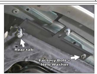
Attach the mounting bracket to the car using the factory bolt, and (1) 3/8'' flat washer in the forward location. Attach the rear tab using (1) 3/8''-16x1 3/4'' hex bolt, (2) 3/8 flat washer, (1) nylon spacer, (1) 3/8 lock washer, and (1) 3/8 nut.
