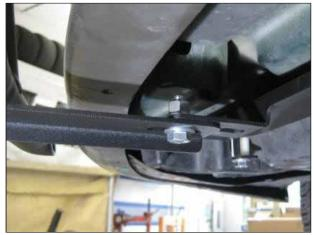
Attach the light bar to mounting bracket using (1) 3/8"-16x 1" hex bolt, (2) 3/8" flat washer, (1) 3/8" lock washer, and (1) 3/8" nut for each side.
