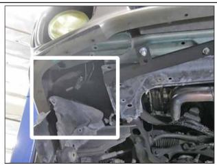
Note: Factory splash guards may need to be partially removed to gain access to the mounting point on the lower sub-frame.
