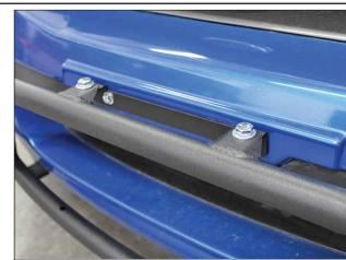
Attach the light bar to License Plate Bracket using (1) 3/8"-16x 1" hex bolt, (2) flat washer, (1) lock washer, and (1) 3/8" nut for each side. Tighten all 3/8" hex bolt to 33 ft-lb.
