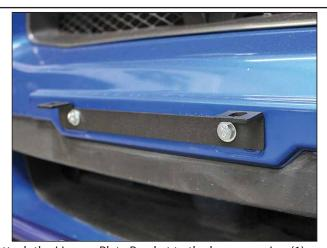
Attach the License Plate Bracket to the bumper using (1) 1/4" Lag Screw and (1) 1/4" Flat Washer for each mounting hole.
