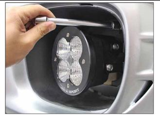
Remove fog light mounting bracket from the vehicle and fasten the new fog light onto it. Install the new fog light assembly onto the vehicle using (1) #10 screw and (3) M6 hex head bolts. Repeat steps on the other side.
