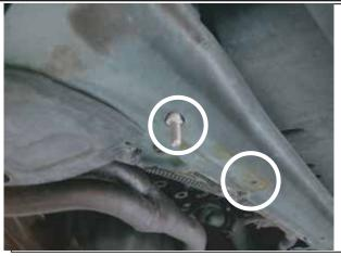
Locate the two holes in the lower radiator support, and place the 5/16" bolt plate into the non-threaded hole [Passenger side shown]
