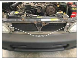
Undo the bolts in between the headlight mounting bolts remove them along with the spacers.
