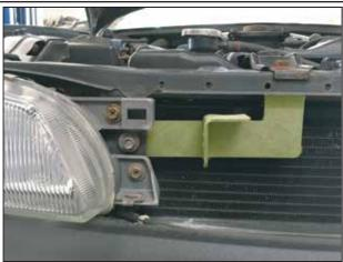
Slide the passenger side upper mounting bracket behind the front of the car as pictured above & reinstall the factory bolts & spacers.
