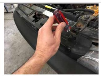
Remove the front grill by pushing down on the release tabs with a flat head screw driver.
