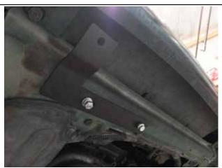
Attach the mounting bracket to the car using the M8-1.25 x25mm bolt, and (1) 5/16 flat washer, (1) 5/16 lock washer, and (1) 5/16 nut fastened on the bolt plate.
