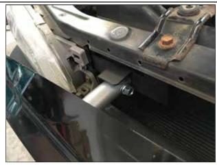
Align the upper mounting brackets with the holes in the the upper tubes & fasten using a (1) 3/8"-16 x 2" Bolt, (2) 3/8" Flat Washers, (1) 3/8" Lock Washer, & 3/8" Nut per side.
