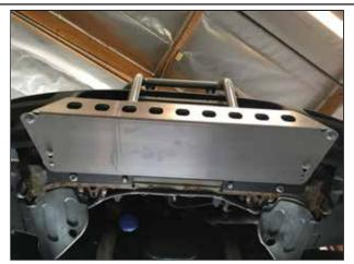
Fasten the front of the Rally Skid Guard to the light bar using (1) 3/8"-16 x 3/4", (1) 3/8" Flat Washer, & (1) 3/8" Lock Washer per side . Tighten all hardware and reattach the front grill.
