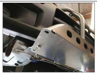
Attach the Rally Skid Guard to the lower mounting brackets using (1) 3/8"-16 x 1" Bolt, (2) 3/8" Washers, (1) 3/8" Flat Washer, & (1) 3/8" Nut on each side, but do not tighten.
