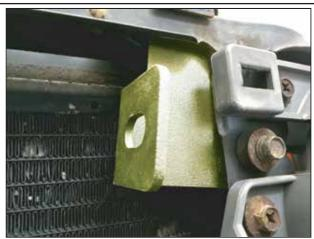
Install the The driver side upper mount bracket using the factory bolt and spacer as pictured above.
