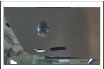
Attach the Skid Guard to the frame using (1) 3/8" washer, (1) 3/8" lock washer, and (1) 3/8" nut per side. Torque 3/8" hardware to 32 ft-lb.
