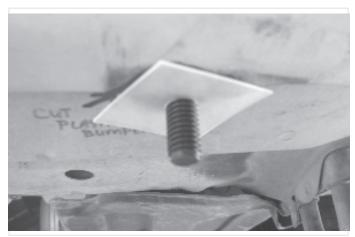
The threaded part of the bolt plate should be sticking through the bottom. Note: Installation may be easier with retaining washer (Not Supllied) 4
