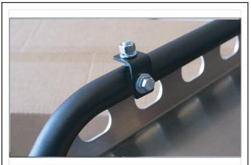
Attach the fog/driving light base to the light bar with the L tab facing forward.
