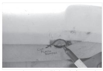
Locate a large and small hole in the frame under the bumper cover. You may need to trim to allow clearance.
