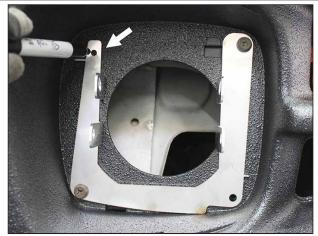
Mount the fog light bracket to the bumper temporarily (using M6 hex head bolts) to mark the additional mounting hole for drilling (use 9/64" drill bit).
