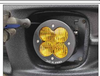
Remove fog light mounting bracket from the vehicle and fasten the new fog light onto it. Install the new fog light assembly onto the vehicle using (1) #10 screw and (3) M6 hex head bolts. Repeat steps on the other side.
