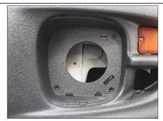
Remove factory fog light and fog light splash guard to gain access to fog light area behind front bumper.
