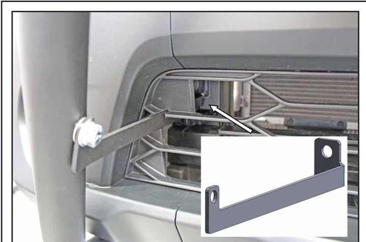
Note the orientation of the upper bracket as shown above. Passenger side shown.
