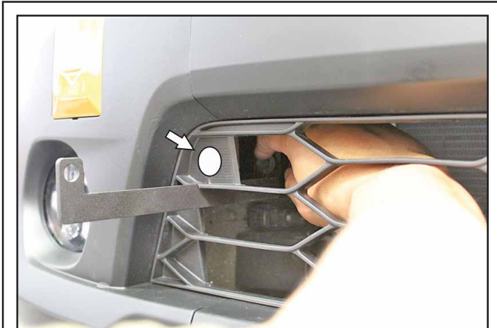
Attach the upper brackets using the factory M6 (10mm head) bolts. Optional: If too difficult to do as shown, cut a hole into the grille panel large enough to insert an extension to fasten the bolt (circle shown).
