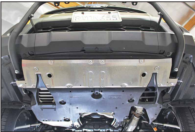
Engine splash shield installed.
