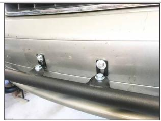
L-bracket installation (continued): Light bar mounting tab will line up over the L-bracket as shown. Fasten using (1) 3/8"-16x1 Hex Bolt, (2) 3/8"Washers, (1) 3/8"Lock Washer, and (1) 3/8"-16 Hex Nut on each side.
