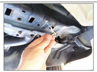
Remove the plastic splash guard. Insert (2) 5/16" Bolt Plates into the holes shown above.
