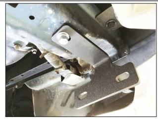
Attach a Mounting Bracket to the Bolt Plates, for each side. Fasten with (1) 5/16" Flat Washer, (1) 5/16" Lock Washer, and (1) 5/16"-18 Hex Nut per side. Note the orientation of the Mounting Bracket with the shorter end pointing forward.
