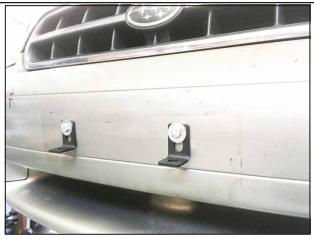
Install L-bracket as shown, with the slotted side mounted on the bumper. Slotted hole - Use  $1/4'' \times 1'' \text{ Lag Screw}$  and 1/4'' USS Washer to mount into the bumper.
