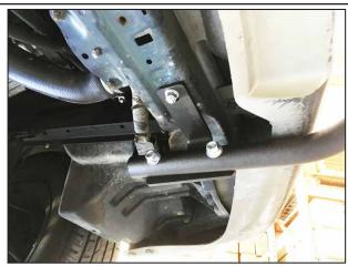
Attach the Light Bar to the Mounting Bracket using (2) 3/8" x 2" Hex Bolt, (4) Flat Washers, (2) Lock Washer, and (2) Hex Nut per side.
