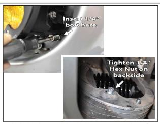
Set aside the bracket and drill out holes to 7/64". Install new fog light onto the mounting bracket. Insert (1) 1/4"-20 Hex Bolt and (1) 1/4" Flat Washer into the small slot on the bracket. Fasten on the back side with (1) 1/4" Flat Washer and (1) 1/4" Kep Nut.
