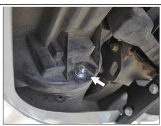
Reinstall the splash guard onto the new bolt and fasten with (1) 3/8" Flat Washer, 3/8" Split Lock Washer, and 3/8" Hex Nut.
