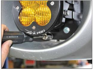
Next, insert (1) 3/8" Hex Head Bolt and (1) 3/8" Flat Washer into the large hole on the bottom of the bracket.
