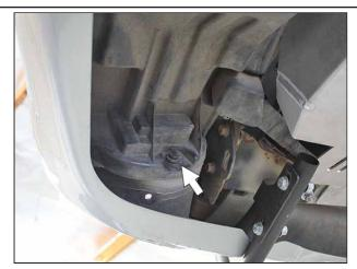
Remove fog light splash guard by unfastening the plastic clip securing it and pulling it downward.
