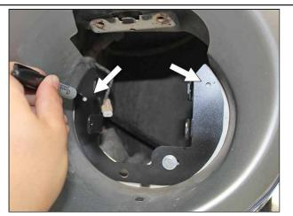
Take the driver side mounting bracket and place it on the mounting surface in the fog light hole. Note the mounting hole locations and align them. Mark the holes located on the sides of the bracket with a pen.
