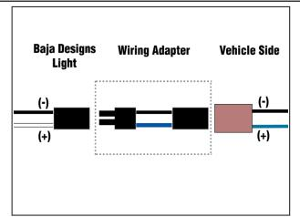
**Wiring:** Now is a good time to do wiring work to adapt the connection of the new light.
