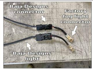
The "new" pair of wiring adapters ready to plug directly into the vehicle harness.
