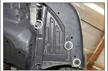
Carefully remove the plastic fasteners to gain access to the area behind the foglight.
