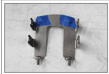
Insert (2) Carriage Bolts into the square holes at the top of the brackets like shown. Ensure the bolts don't fall out by taping the heads to the bracket.
