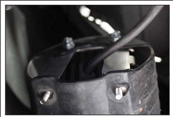
Insert the foglight assembly in the reverse order as the removal of the factory light. It may take a few tries but the top two bolts should slide through the factory holes and then you can fasten them down using (1) 1/4" Flat Washer, (1) Lock Washer and (1) Hex Nut on each bolt.
