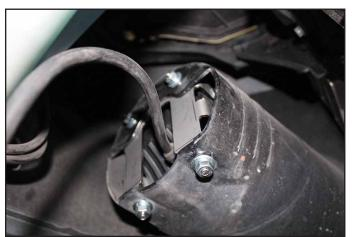
Insert (2) Carriage Bolts in the bottom holes in the fog light bracket through the open space behind the fog light. Fasten them using (1) 1/4" Flat Washer, (1) Lock Washer, and (1) Hex Nut.
