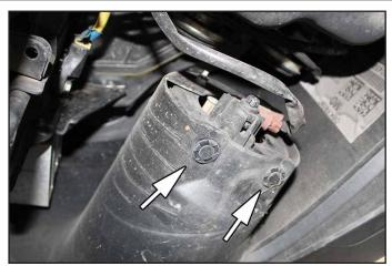
Carefully remove (2) plastic rivets from the fog light cover to release the bottom of the fog light.
