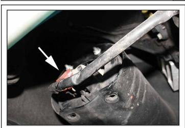
Unplug the foglight by depressing the tab on the connector and carefully sliding the connector off.
