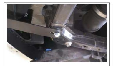
Attach the lower bracket to the lower sub-frame using (1) 3/8"-18 x 3" hex bolt & (1) nut on each side. The threaded portion should point upward.
