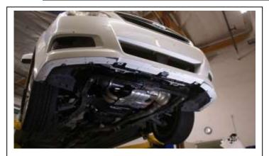
After securely lifting the vehicle, remove the factory center splash guard.
