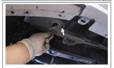
Feed the 5/16" bolt plate (aluminum side) into the larger opening on the lower radiator support. The threaded bolt should stick out of the hole that the arrow is pointing to.
