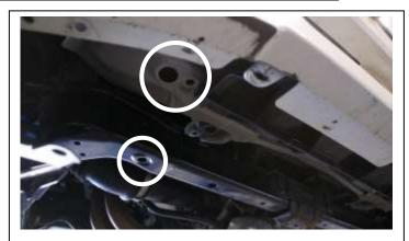
Locate the two mounting locations for each lower bracket. The location is at the lower radiator support and front sub-frame.
