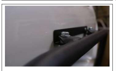
Attach the upper portion of the light bar using the supplied 3/8" nylon spacer, (1)3/8"-18 x 1 ½" hex bolt, (2) 3/8 flat washer, 3/8 lock nut, and 3/8 nut on each side. **Keep loose for adjustments**.
