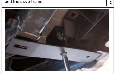
Attach the bracket to the lower radiator support. **Note:** Insert the ratchet extension into the through hole, then attach the 7/16" Socket.
