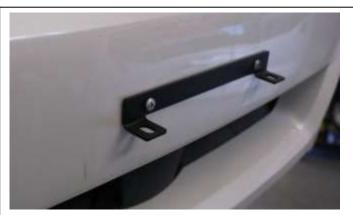
Attach the upper bracket using the stock license plate screws. **Do NOT overtighten** as it may strip the plastic threads.
