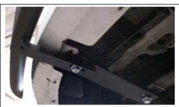
Attach the lower portion of the light bar using the supplied 3/8"-18 x 1" hex bolt, (2) flat washer, (1) lock washer, and 3/8 nut on each side. Verify light bar fitment, then tighten all hardware.
