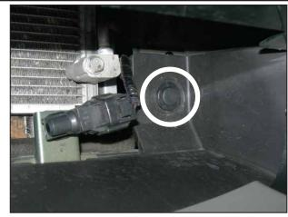
Remove the (2) plastic clips shown located inside the lower air dam.
