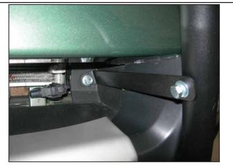
Fasten the (2) Upper Brackets to the bar with (1) 5/16" x 1" Hex Bolt, Lock Washer, and Flat Washer each. Fasten the rear bolt with (1) Flat Washer, Lock Washer, and Hex Nut.
