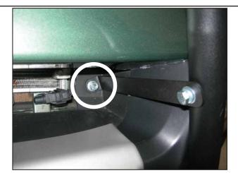
**For 2013-14 Outback:** Use 5/16" x 1.5" Hex Bolt and insert 3/4" Spacer in front of the hole shown.
