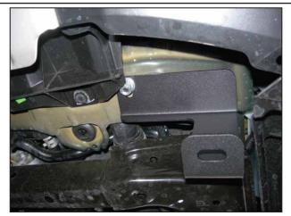
Attach (2) Lower Brackets to the Bolt Plates. Fasten with (1) 3/8" Flat Washer, Lock Washer, and Hex Nut per side.
