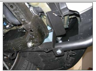
Attach the Bar to the Lower Brackets using (1) 3/8" x 2.5" Hex Bolt, (2) Flat Washers, (1) Lock Washer, and (1) Hex Nut per side.
