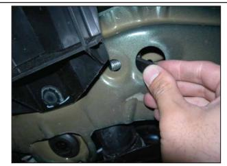
Remove the plastic splash guard. Insert (2) 3/8" Bolt Plates into the holes shown above.
