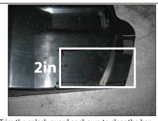
Trim the splash guard as shown to clear the bar and re-attach.
