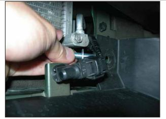
Insert (1) 5/16" x 1" Hex Bolt and Flat Washer into the holes shown.
