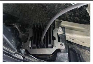
Install the new foglight assembly onto the bumper using M6 bolt and washer from previous step.
