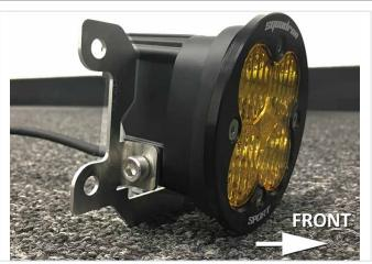
Attach new foglight to Light Conversion Bracket like shown above. Repeat on passenger side.
