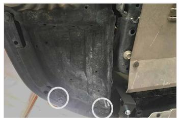
Remove the plastic rivets from the driverside splash guard to access the foglight area (keep for later). Repeat on the passenger side.
