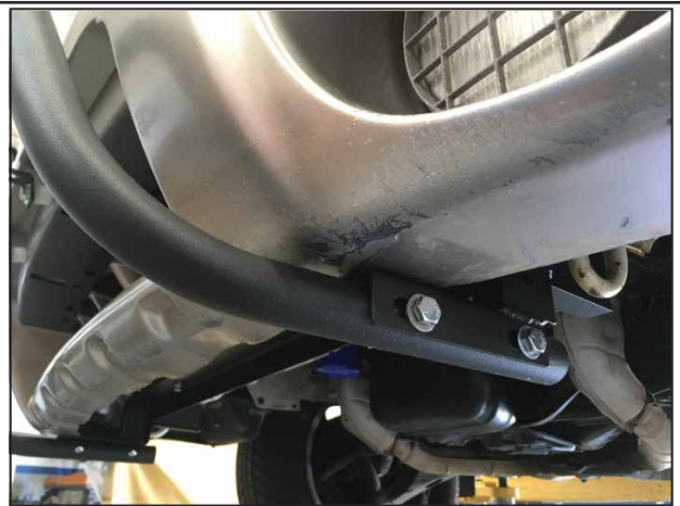
Additional view from Step 7. Note there are also Flat Washers on the other side of the mounting brace. Once Light Bar is in place, tighten and torque 3/8" hardware to 30 ft lbs.
