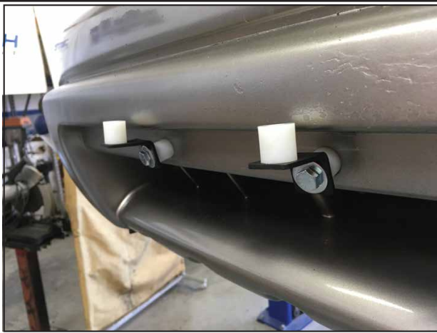
Position plastic spacers on top of "L" Brackets as shown.
