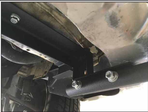
Attach the Light Bar to the Mounting Bracket using (2) 3/8" x 2" Hex Bolt, (4) Flat Washers, (2) Split Lock Washers, and (2) Hex Nuts per side.
