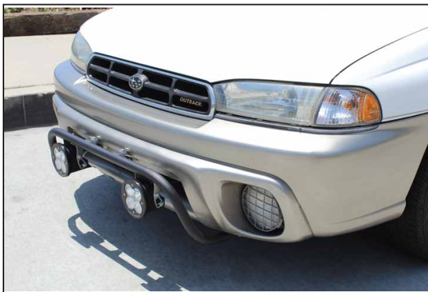
Finished install of the light bar. Baja Designs XL-R lights are shown.
