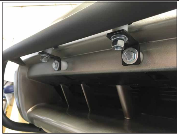
Place Light Bar on top of plastic spacers. Use (1) 3/8"-16x1 Hex Bolt, (2) 3/8" Washers, (1) 3/8" Split Lock Washer, and (1) 3/8"-16 Hex Nut. Assemble loosely.
