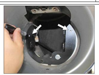
Take the driver side mounting bracket and place it on the mounting surface in the fog light hole. Note the mounting hole locations and align them. Mark the holes located on the sides of the bracket with a pen.
