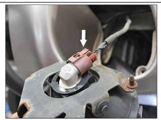
Unplug the light from the harness by depressing the tab on the back.
