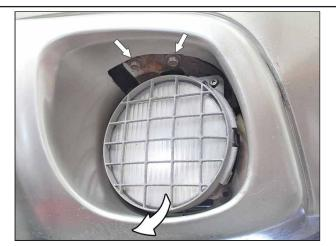
Remove factory fog lights from the front bumper by undoing the (2) factory bolts and pull down and out.
