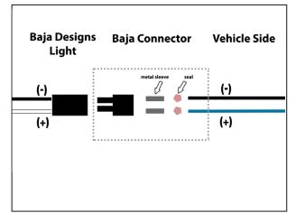
**Wiring:** Now is a good time to do wiring work to adapt the connection of the new light.
