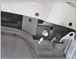
Attach the mounting brace to the lower bumper beam by using (1) 3/8" Flat Washer, (1) 3/8" Lock Washer, (1) 3/8"-16 Hex Nut. Repeat on the opposite side.
