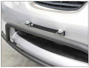
Attach the light bar to License Plate Bracket using (1) 3/8"-16x 1" Hex Bolt, (2) Flat Washer, (1) Lock Washer, and (1) 3/8" Hex Nut for each side.
