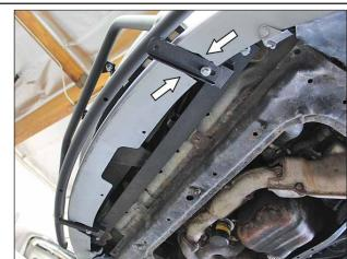
Attach the light bar to the lower brace using (1) 3/8"-16x 1", (1) 3/8" Lock Washer, and (1) 3/8" Flat Washer on each side. Tighten all 3/8" hardware to 33 ft-lbs. Trim bumper as needed to clear the light bar mounting to the brace (shown with arrows).
