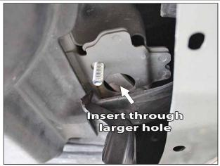
Insert the bolt plate through the larger hole and have the threads come out of the smaller hole like shown above.
