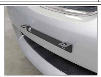
Attach the License Plate Bracket to the bumper using (1) 1/4" Lag Screw and (1) 1/4" Flat Washer in each mounting hole to the factory location.
