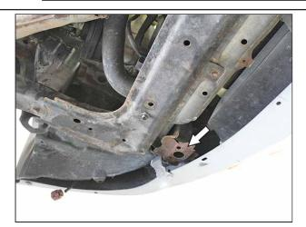
Remove the factory splash guard. Locate holes (shown above) on lower bumper beam. There is one on each side (L+R) of the car.
