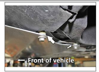
Carefully raise the plate against the vehicle, aligning the holes with the holes on the vehicle. Ensure the spacers are properly aligned so that each new M8x40mm Flange Head bolt inserts through them and into the vehicle.
