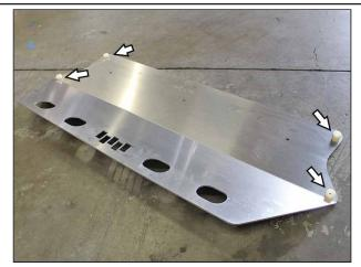
Place the included round spacers over each mounting hole on top side of the new skid plate.
