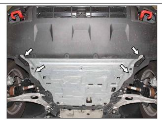
Locate and remove the (4) M8 Hex Head bolts shown above which are fastened to the factory skid plate. They will be replaced with the included longer M8 Flange Head bolts later.
