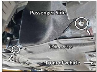
Locate and remove the (1) M8 Hex Head bolt & (1) M10 Hex Head bolt (rear) underneath the front of the vehicle. Passenger side shown.
