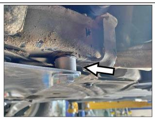
Place the 5/8" spacers between the rear-most holes on the skid plate and the chassis. Insert the new M10 Bolts into the holes and thread them into the chassis. Orientation: (1) M10 Bolt, (1) M10 Washer, skid plate, short spacer.
