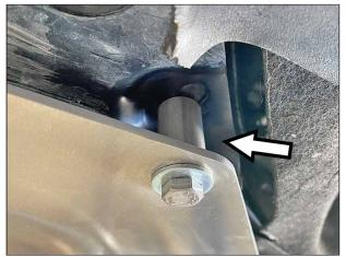
Place the 1.25" round spacers between the front holes on the skid plate and the chassis. Insert the new M8 Bolts into the front holes and thread them into the chassis. Orientation: (1) M8 Bolt, (1) M8 Washer, skid plate, long spacer.
