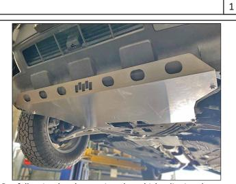
Carefully raise the plate against the vehicle, aligning the holes with the holes on the vehicle.
