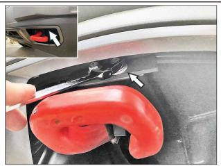
Locate and remove the (outer) tow hook bolt shown above. (Driver side pictured). Loosen the bolt next to it but, do not remove. Repeat step on the passenger side.
