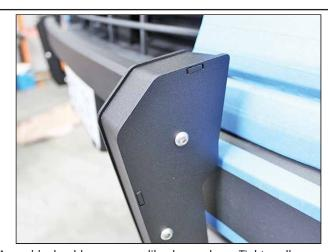
Assembly should now appear like shown above. Tighten all hardware, including the bolts securing the mount to the tow hook area behind the bumper.
