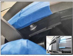
Once the mounting bracket is in position, reinstall the other bolt but keep them loose to allow the mounting bracket to move around during installation of the rest of the assembly. Repeat on passenger side.
