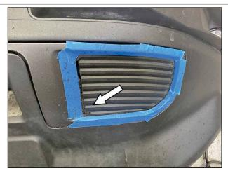
Take extra caution around the inner-bottom corner shown above because there is a structure behind it you don't want to accidentally cut into (cutting the bumper while off the car can help prevent this altogether, however it is a lot more work).
