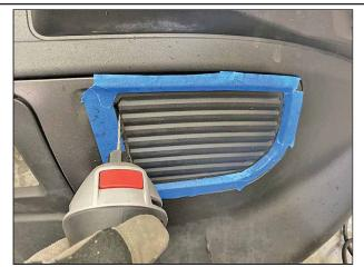
Locate and cut out the tow hook holes in the front bumper cover. A dremel tool works great to get a clean cut. (Skip to step 4 and refer to Addendum if your vehicle comes equipped with Front Tow Hooks)
