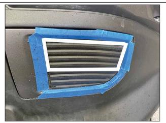
Side note: If you want to leave some material on the bumper cover (if you will not be installing tow hooks, for example) you can potentially cut about 2/3 of the rectangle area out instead. Once the holes are cut-out you can reinstall the bumper cover to the vehicle and begin installing the Chassis Mounting Brackets.
