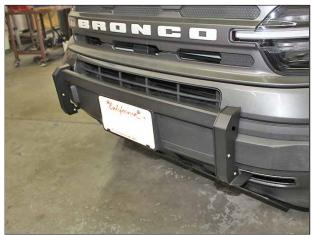
Fit the light bar assembly carefully between the mounts. Have a friend help out as it can be a bit tricky to do on your own. **Tip:** Loosening the bolts on the Chassis Mounting Brackets can aid in fitting it in.
