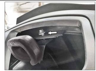
Ensure the adjacent bolt is loosened roughly 1/4" to allow room for the mounting bracket to slide between it and the chassis.
