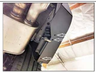
After aligning the splitter, use the (3) splitter holes to mark the centerline holes for drilling.
