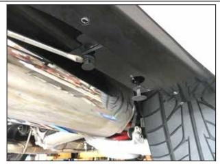
Remove (2) large plastic rivets that hold the bumper to a plastic structure to allow easier access for installation.
