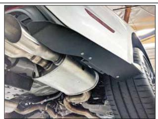
Fasten the 3 holes with (1) 5/16"-18x1.00" Buttonhead Bolt, (1) Flat Washer, (1) Lock Washer, and (1) Hex Nut on each hole.
