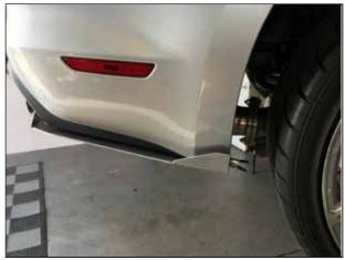
Align the front edge of the splitter to the wheel arc. Use holding clips to help keep the splitter in place temporarily.
