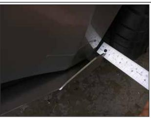
Confirm that both left and right splitter are consistent in alignment (fin, bumper outline, and exhaust clearance).
