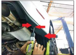
After confirming alignment of the rear splitter and marking the holes, drill the (3) holes with a 3/8" drill bit.
