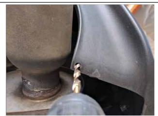
**Premium Version**: Rear-most hole, Drill with a 3/8" drill bit.
