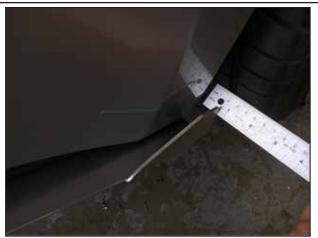
Confirm that both left and right splitter are consistent in alignment (fin, bumper outline, and exhaust clearance).
