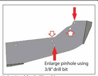
Holes Used for Drilling Diagram:
