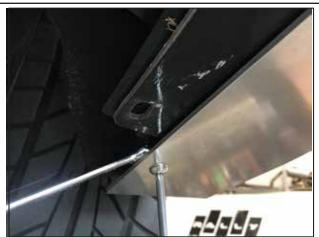
Fasten the two forward-most holes with (1) 5/16"-18x1.00" Buttonhead Bolt, (1) Flat Washer, (1) Lock Washer, and (1) Hex Nut on each hole. Fasten rear hole using (1) 5/16"-18x1.00" Buttonhead Bolt, (1) Flat Washer, (1) Lock Washer, and (1) Hex Nut Reattach the plastic rivets.
