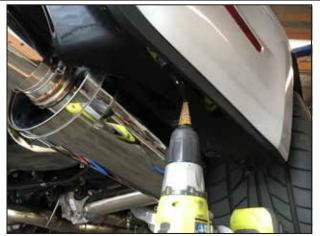
Using the provided diagram for reference shown below, Drill the (3) holes with a 3/8" drill bit. (Premium bumper: Confirm corner of bumper near exhuast lines up to drill the rear-most hole)
