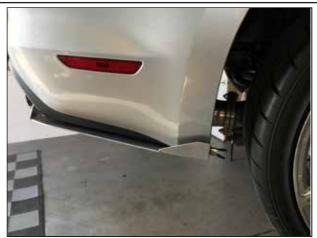
Align the front edge of the splitter to the wheel arc.
