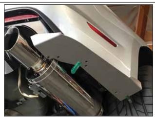
After aligning the splitter, use the (3) splitter holes to mark the centerline holes for drilling. Refer to diagram provided, for the holes used in NON-PREMIUM versus PREMIUM rear bumper versions.
