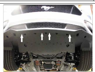
Find the (4) corresponding OEM clip-on nut hiding behind the OEM front splitter, as indicated above by the (4) arrows. These are the attachment points for the center splitter.
