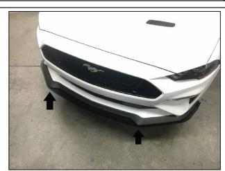
Confirm alignment of the 3 splitter pieces, and tighten all hardware.
