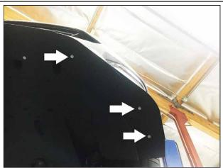
Fasten the side pieces using the 3 points, with the (2) OEM screws, and (1) #8 x 1.5" Screw and (1) #8 washer. Loosely tighten, to allow for adjustments.
