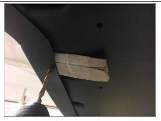
Drill out the (4) holes for the center piece, and (2) total holes for the side pieces using a pilot hole and 5/16 drill bit. Tip: Place a thin block of wood or layers of cardboard behind the OEM splitter, as shown above.
