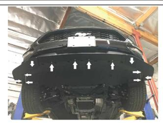
Make sure the center piece is ON TOP of the side pieces. Confirm final alignment and tighten all hardware.
