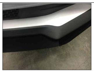
After marking the (4) holes for the center piece, and (2) total holes for the side pieces, confirm the markings by aligning the center and side splitter pieces to the marked holes. Check splitter alignment.
