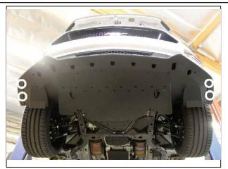
**GT Version (For Non-GT, see page 4 and 5):** Remove the (4) OEM screws holding the OEM splitter, as shown above with circles.
