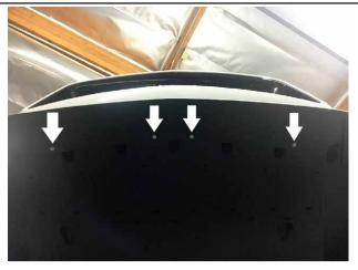
Re-install the clip-on nuts, and slide the center piece back ON TOP of the side pieces. Fasten the center piece using the (4) points, each with (1) #8 x 3/4" Screw and (1) #8 washer. Loosely tighten, to allow for adjusments.
