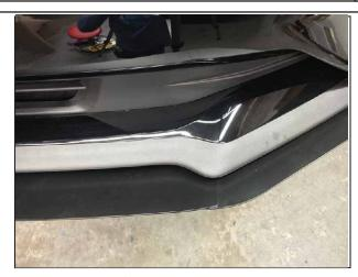
Check alignment of the side and center piece.
