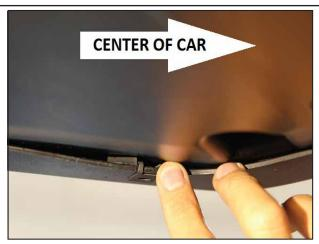
Attach (1) clip-on nut, per side, as shown above. The driver (left) side is shown. Note the OEM plastic rib on the OEM splitter is used to place THE clip-on nut against it. Mark the centerpoint of the hole.
