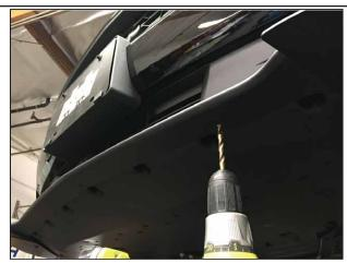
Drill the (4) holes for the center piece. Drill bit should be able to go through 1/2" deep, through 2 layers of plastic (the bumper trim and the splash guard).
