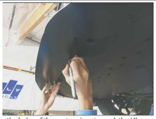
Use the holes of the center piece to mark the (4) preliminary drill locations on the OEM bumper. Remove the center piece.
