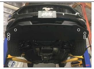
Non-GT Version (For GT, see page 1 and 2): Remove the (8) OEM screws as indicated above in circles.
