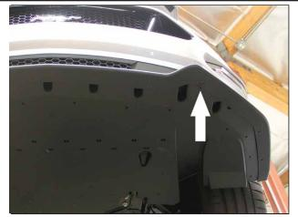
Locate the plastic rib in the area shown above, and attach a clip-on nut on each side. Place clip-on nut on the center side of the rib (i.e. inward to center of car).
