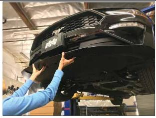
Confirm the placement of the clip-on nuts by sliding the center piece back ON TOP of the side pieces. Double check the holes, side piece, and center alignment. Re-adjust clip-on locations by sliding in small increments. Recheck alignment, and mark final drill locations. Remove clip-on nuts to prepare for drilling.
