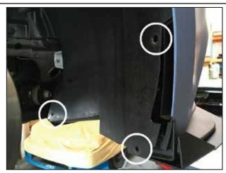
**(GTPP and Non-GTPP)** Remove the indicated fenderliner clips and pry the liner away to access the inside of the bumper cover.
