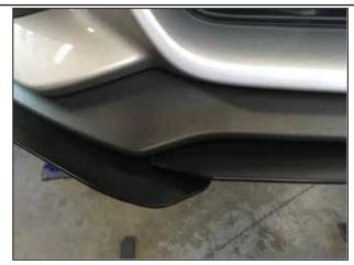
(Non-GTPP) Check that the center piece rests on top of the side pieces. Adjust fitment and tighten all hardware.
