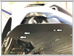
**(GTPP)** Attach Side Piece with (2) Factory Screws, and (1) #8 x 1.5" Screw, (1) #8 Washer, and (1) 1/4" Washer on each side.
