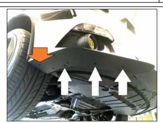
(Non-GTPP) Remove the indicated screws (3 long arrows) from the factory splitter. Loosely attach side pieces with factory screws. Note: Short arrow (left most arrow) will be used to drill
