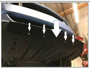
(GTPP) Attach the Center Piece with (1) Factory Screw [as indicated by large arrow], and (4) #8 x 1.5" Screws, (4) #8 Flat Washers, and (4) 1/4" Flat Washers [as shown by 4 smaller arrows]
