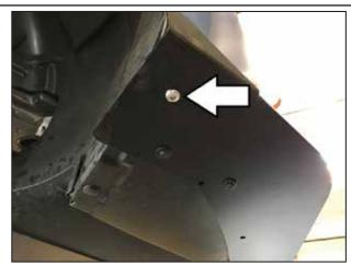
(GTPP and Non-GTPP) Fasten with (1) 5/16" Buttonhead Screw, (1) Flat Washer, (1) Lock Washer, and (1) Hex Nut per side. Reattach the fender liner.
