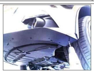
(Non-GTPP) Drill the indicated hole through the bumper with a 5/16" Drill Bit, per side.
