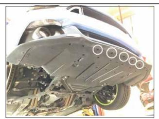
(GTPP) Remove the (5) indicated screws.
