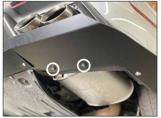
While holding up the passenger side splitter piece against the rear bumper, fasten the factory bolts that affix to the rear mounting hole locations here.
