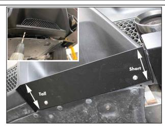
Use a 5/16" drill bit to drill the mounting holes, once marked. Attach the corresponding center piece as shown. Note: The passenger side center piece is wider towards the center of the car and narrower towards the outside of the car. The driver side is the opposite. Use a 5/16-18 x1" Buttonhead Bolt, Flat Washer, Split Lock Washer, and Hex Nut for each of the holes.
