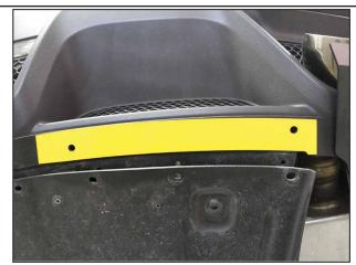
Use the included template to mark the holes for drilling on the rear bumper.
