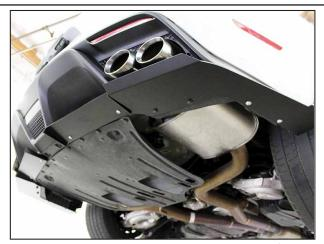
Repeat previous steps on the opposite side. Return factory fasteners to their respective locations to reattach the rear diffuser and inner bumper support structure on both sides.
