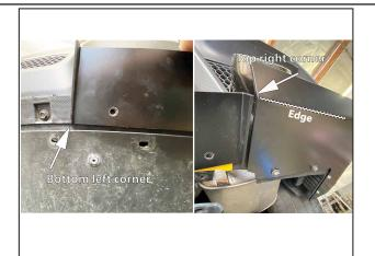
While holding the Center Splitter up, align the top right corner with the bend edge on the Side Splitter. Also, align the bottom left corner with the edge of the bumper, as shown.
