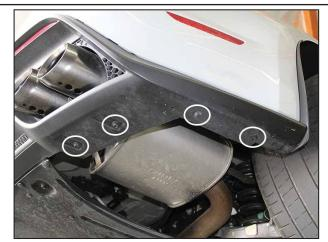
Remove factory plastic fasteners and 10mm hex head
