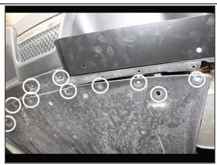
Next remove the factory plastic fasteners and 10mm hex head bolts from the rear mounting locations of the rear diffuser panel. Doing this aids in gaining access behind the mounting hole locations to fasten the hex nuts to the bolts
