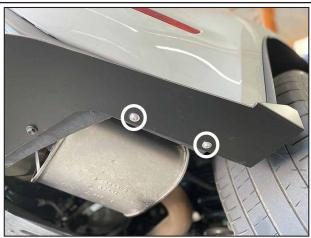
Insert a 1/4-20 Sockethead Bolt with a 1/4" Flat Washer into each of these mounting holes. On the opposite end of each bolt affix another 1/4" Flat Washer, followed by a 1/4" Split Lock Washer and Hex Nut. Tighten down all hardware.
