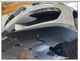
Attach the side splitter with a 5/16-18x1" Buttonhead Bolt, 5/16" SAE Flat Washer, Split Lock Washer, and Hex Nut in each hole. Repeat on the opposite side splitter. Keep the bolts loose for now.
