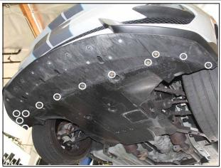
Remove the torx screws located underneath the front bumper, affixing the splash guard to the car. This step aids in gaining access behind the cover to fasten the mounting hardware in later steps.
