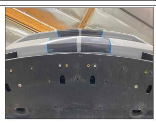
Drill the Center Splitter holes using the 13/32" drill bit. Install the Rivnuts in the newly drilled holes using the method shown in the following steps.
