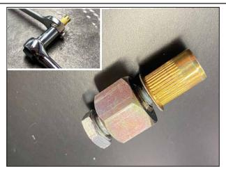
**Rivnut Installation:** Take your Rivnut Tool Kit and thread it onto the Rivnut like shown. Use a 9/16" Wrench to hold the collar and 7/16" Socket Wrench to tighten down the Rivnut. Be careful not to overtighten. This step requires some patience to install properly.
