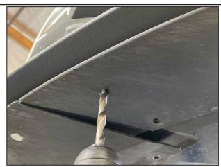
Remove the Center Splitter and set aside. With the Side Splitter still attached to the vehicle, carefully swing it out of the way to begin drilling the newly marked holes. Use a 5/16" drill bit to drill out the (2) new holes on the splash guard.
