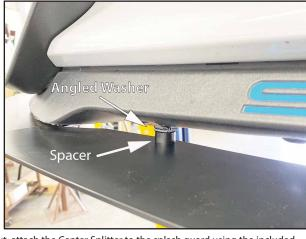
Next, attach the Center Splitter to the splash guard using the included 1/4-20 x 1.25" Buttonhead Bolts. Place (1) Angled Washer and (1) 3/8" Spacer in between the splitter and the splash guard for each mounting hole. Keep hardware loose until you fasten the Bind Post Screws in Step 14.
