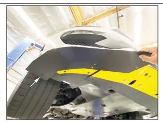
Once you have all the templates on the splash guard, find the (2) side splitters and loosely reinstall them on the car with the factory 7mm head screws removed in step 1.
