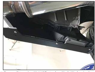
Install rear splitter using (1) 1/4" Buttonhead bolt, Washer, Lock Washer, and Hex Nut on the rear most mounting hole. Install (2) 5/16" Buttonhead bolts, Washers, Lock Washers, and Hex Nuts on the remaining mounting holes. Reinstall plastic rivets and screws removed in steps 1-2.
