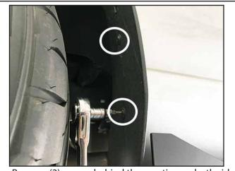
Remove (2) screws behind the rear tire, on both sides of the vehicle.
