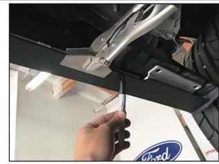
After aligning the splitter, use the (3) splitter holes to mark the centerline holes for drilling. The rear-most hole may already exist in the bumper and does not require any drilling.
