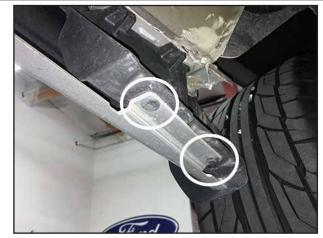
Remove the (2) plastic rivets that hold the bumper to a plastic structure on both sides of the vehicle.
