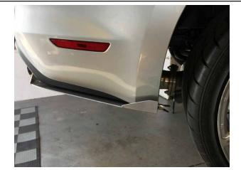
Hold the splitter up to the bumper and ensure the front of the splitter seats flush with the arc of the wheel well.
