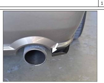
Align the rear fin with the exhaust cutout curve on the bumper.
