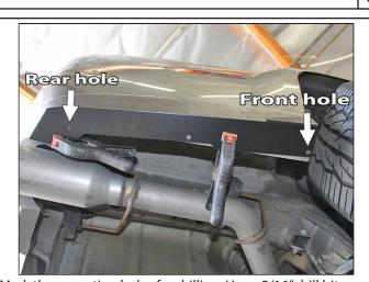
Mark the mounting holes for drilling. Use a 5/16" drill bit for the front and center holes. Use a 1/4" drill bit for the rear-most hole.
