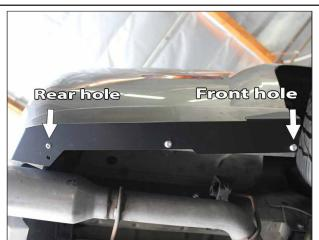
Fasten (1) 5/16"-18 Buttonhead Bolt, (1) 5/16" Flat Washer, (1) 5/16" Split Lock Washer, and (1) 5/16"-18 Hex Nut to the front and center holes. Fasten (1) 1/4"-20 Buttonhead Bolt, (1) 1/4" Flat Washer, (1) 1/4" Split Lock Washer, and (1) 1/4"-20 Hex Nut to the rear-most hole.
