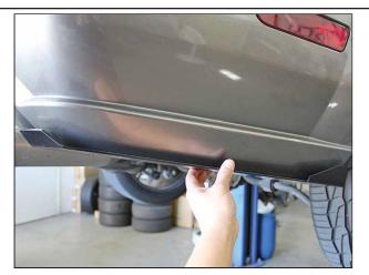
Hold up the passenger side splitter piece to the bumper.
