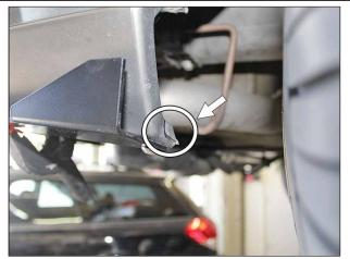
Mark this portion of the rear bumper to be cut-out. Carefully cut out the piece.
