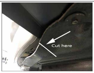
The sides of the splashguard will need to be tucked into the bumper cover. Cut a relief line through the splashguard, parallel to the edge of the center splitter, as shown above. Then, tuck the loose hanging portion up and into the bumper cover.
