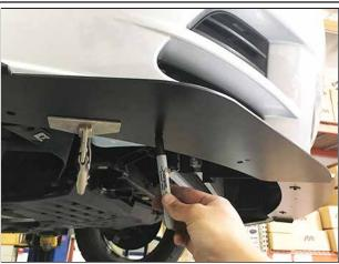
Place the side splitter up against the front bumper cover, lieing underneath the corner of the center splitter. Line the side splitter up with the center splitter, then mark the drill holes for mounting the side splitter.
