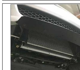
Mount the center front splitter loosely to the front bumper cover using the original screws and clip-nuts. In the next step, the center splitter is used as a reference to mount the sides.
