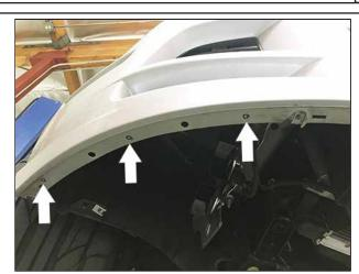
Confirm your marks on the front bumper and drill out holes to 5/16" (start with a smaller size drill bit, i.e. 1/8" or similar, as a pilot hole).
