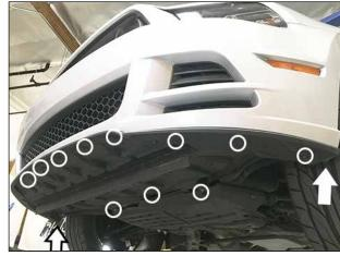
Remove the 7mm hex head screws. Note, there are also two screws located in the wheel wells on either side of the car directly behind the front bumper cover (see arrows). These will need to be removed as well (they will not be reused).
