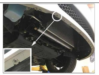
Retain the factory clip-nuts on the bumper cover. These will be reused to mount the front splitter.
