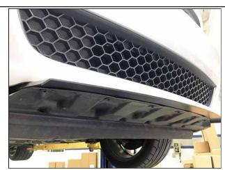
Reattach splashguard in the opposite manner as removal except now with the front portion lieing underneath the center splitter. (Remove the screws attached in step 8 and reattach them underneath the splashguard, sandwiching the center splitter to the bumper cover like shown above.)
