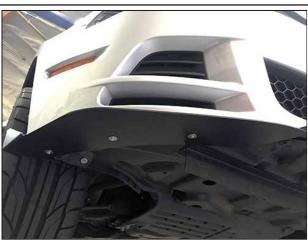
Attach the side splitter using the included #8 screws and washers. Repeat steps 9-10 to mount the opposite side splitter. Ensure all hardware is tightened down. Installation is complete.
