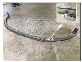
Finally, release the front chin spoiler by depressing the tabs shown above with a flathead screwdriver.
