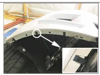
Place the included clip-nuts over the new holes with the flat side facing down.
