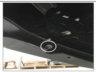
Remove the remaining screws on each side of the chin spoiler.
