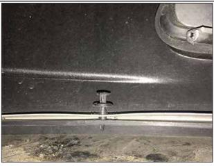
Remove the plastic clips, (3) on each side, using a flathead screwdriver.
