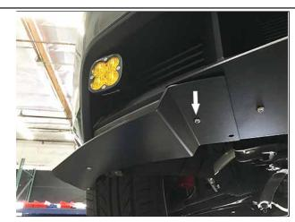
Attach side splitter with (1) 5/16"-18 x1.00" Buttonhead bolt, (1) 5/16" Washer, (1) 5/16" Lock Washer and (1) 5/16"-18 Hex Nut in the hole shown above.
