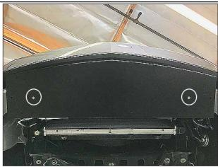
Reattach middle splitter with (2) 5/16" x1.00" Buttonhead bolts, (2) 5/16" Washers, (2) 5/16" Lock Washers, and (2) 5/16"-18 Hex Nuts in the circled holes shown above. Do not tighten all the way yet.
