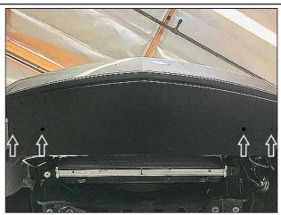
You should have marked (4) holes for drilling as shown above. Remove the middle splitter and drill out the marked holes with a 3/8" drill bit.
