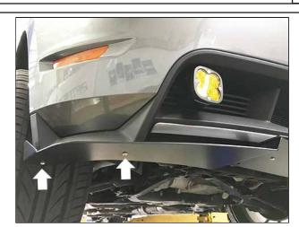
Attach the splitter using (2) 5/16"-18 Buttonhead Bolts, (2) 5/16" Washers, (2) 5/16" Lock Washers, and (2) 5/16"-18 Hex Nuts. Repeat steps 6-10 on the other side.
