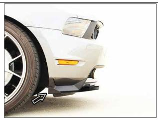
Hold up one of the side splitters to the bumper and align the fin to seat flush with the arc of the wheel well as shown above.
