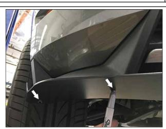
Ensure the fin is still aligned (as shown in step 6) and mark the centerholes for drilling as shown above. Drill out the marked holes with a 3/8" drill bit.
