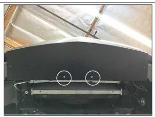
Locate the two center holes on the front bumper and mount the middle splitter piece using (2) #8x1.5"
