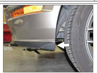
Hold the splitter against the bumper, align the holes with the template and check that the fin on the splitter is collinear with the rear bumper edge. If not, readjust and mark holes. Drill holes out to 1/4". Repeat on passenger side.
