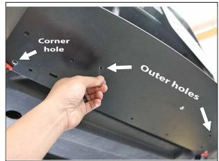
Line up the **corner** holes with the factory mounting holes in the bumper. Mark the two **outer** holes for drilling. Drill out holes to 1/4". Fasten the new holes with hardware in the following orientation: (1) 1/4"-20x1.5" Buttonhead Bolt > Splitter > Spacer > 1/4" Flat Washer, 1/4" Lock Washer, and 1/4" Hex Nut.
