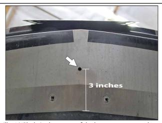
Drill a 1/4" hole in the center of the bumper to mount the center splitter. The hole should be located 3" from the rear edge.
