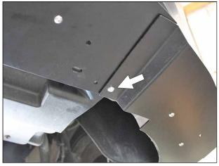
Fasten (1) #8 x 1.5" Screw and (1) #8 Flat Washer to the factory j-clip on the splash guard, securing the splitter pieces together with the bumper.
