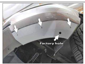
Place the driver-side template onto the bumper like so. Line up the hole in the bumper with the template. The other 3 holes are to be drilled out.
