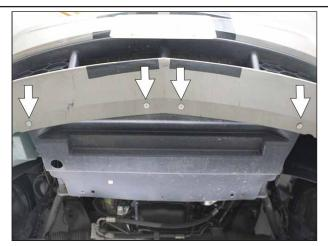
Remove the 4 screws holding the splash guard to the front bumper.
