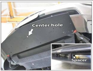
Place (1) Spacer on top of the center hole on the center splitter. Fasten the splitter loosely to the bumper using the supplied hardware in the following orientation: (1) 1/4"-20x1.5"
