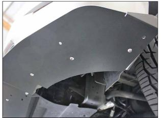
Loosely fasten the side pieces to the bumper using hardware in the following orientation: (1) 1/4"-20x1" Buttonhead Bolt > Splitter > 1/4" Flat Washer, 1/4" Lock Washer, and 1/4" Hex Nut. Do not tighten yet.
