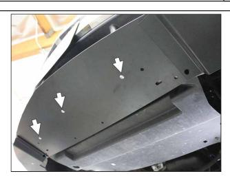
Tighten the (3) bolts securing the center splitter to the bumper using a 5/32 hex key and 7/16" wrench.
