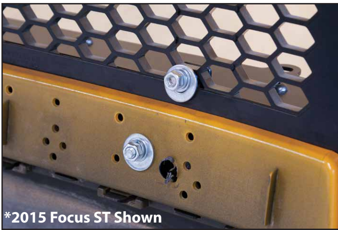
Fasten with 1/2" Flat Washer, 5/16" Flat Washer, 5/16" Lock Washer, and 5/16" Hex Nut.
