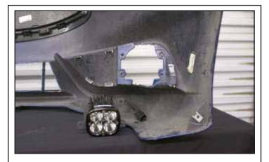
Replace Baja Designs Squadron Brackets with supplied Mounting Brackets. Tighten so that the brackets are parellel to the face of the fog light.
