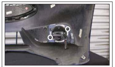
Gain access to the fog lights from behind the bumper. You may pull back the fender liner or remove the bumper entirely.
