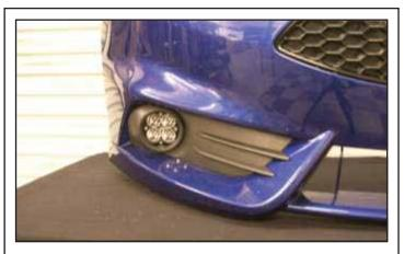
Note: It is normal for a small gap to be present between the lights and bezel.
