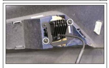
Install the assembly onto the bumper with the OEM screws.
