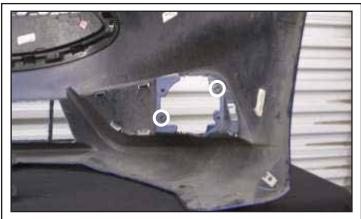
Remove the (2) T25 Torx Screws circled.
