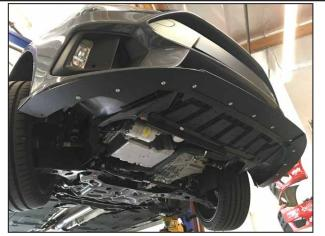
Insert plastic splash guard above the Splitter hardware.
