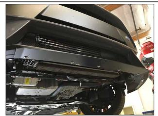
Attach the Center Piece with (5) 1/4" Buttonhead Screws, (10) Flat Washers, (5) Lock Washers, and (5) Hex Nuts.
