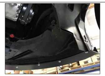
Reach above the splash guard and insert (1) 1/4" Buttonhead Screw, (2) Flat Washers, (1) Lock Washer, and (1) Hex Nut through the last holes.
