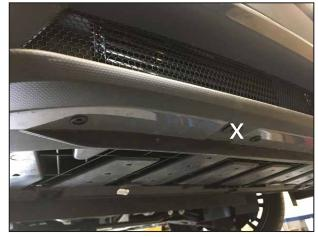
Remove the plastic splash guard. Take note of the overlaps at the wheel well. Ignore the plastic clips indicated with an "X" above.
