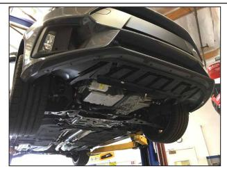
Remove the felt splash guard.
