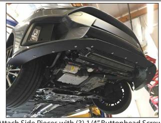
Attach Side Pieces with (3) 1/4" Buttonhead Screws, (6) Flat Washers, (3) Lock Washers, and (3) Hex Nuts on each piece.
