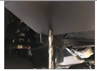
Drill the (2) remaining holes in the Front Splitter through the plastic splash guard with a 5/16" Drill Bit.
