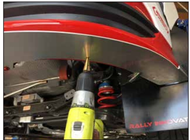
Drill the (2) holes with a 3/8" Drill Bit.
