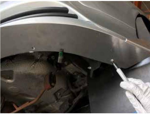
Mark the (2) holes onto the rear bumper cover.
