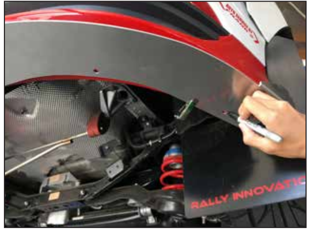
Mark the (2) holes onto the rear bumper cover.
