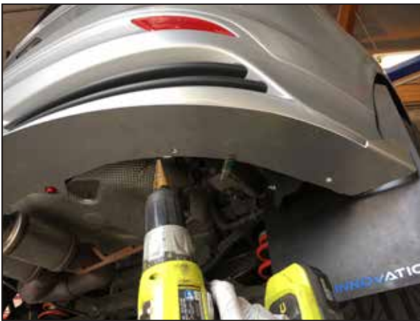
Drill the (2) holes with a 3/8" Drill Bit.
