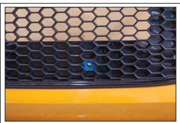
Drill through the centers of the marked hexes with a 3/8" Drill Bit.
