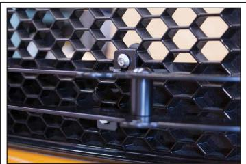
Insert (2) 5/16"-1.25" Buttonhead Screws through the top tabs and (2) 5/16"-1.75" Buttonhead Screws through the bottom tabs.
