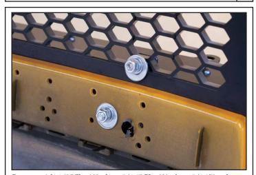
Fasten with 1/2" Flat Washer, 5/16" Flat Washer, 5/16" Lock Washer, and 5/16" Hex Nut on each bolt. Tighten all hardware. Recommend installing lights prior to reinstalling bumper cover.
