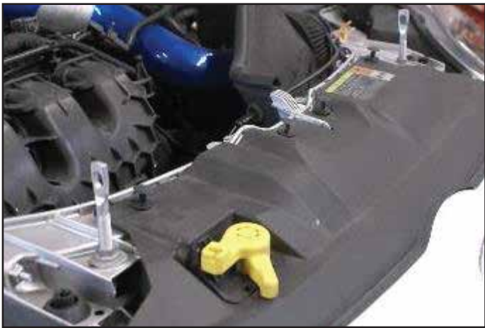
Detach hood release cable and remove front bumper.
