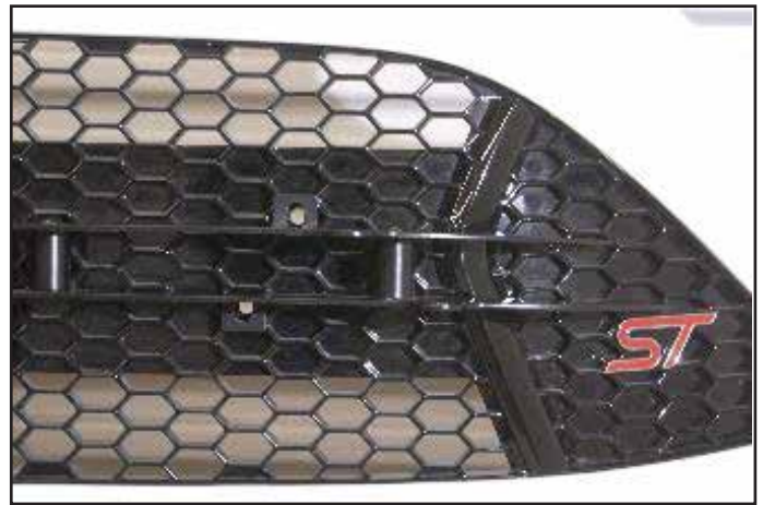
Align light plate to grill as shown above. Take note of hole locations with respect to grill hexes.
