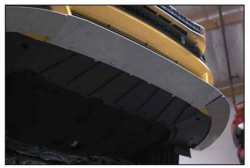
Attach center piece, then side pieces using OEM hardware. Optional: Drill out OEM holes and use supplied 5/16"x1" hardware.
