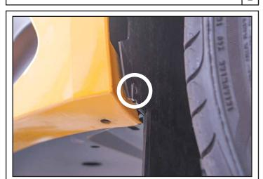
Remove lowermost screw on fender liner and pull away for clearance.
