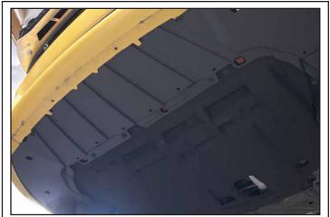
Remove the front splash guard attached to the front bumper.
