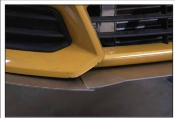
Check that the center piece rests on top of the side pieces. Check alignment on both sides and tighten hardware.
