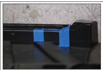
Cut the splash guard on both sides as shown. Extend the cut approximately 1.5" onto the top face.
