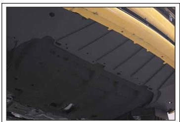
Re-insert splash guard, but do not attach hardware. Reach through the back to insert mounting hardware for the splitter.
