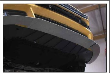
Insert (2) 5/16"x1.25" Buttonhead Screws and secure with Flat Washer, Lock Washer, and Nut. Tighten all hardware.
