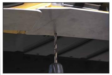
Drill out remaining holes on the center piece with a 3/8" Drill Bit.
