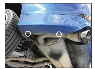
Locate the mounting holes in the rear bumper (circled above). Remove the screws from them.
