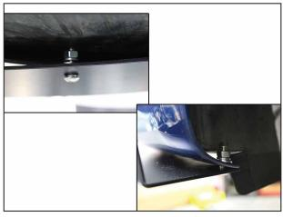
Install 5/16" hardware in the order as follows: Buttonhead bolt, Flat Washer, Split Lock Washer, Hex Nut. Loosely tighten for now.
