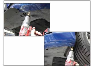
Drill holes out using a step drill bit to 5/16 inch.
