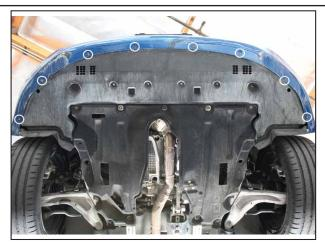
Locate the mounting holes in the front bumper (circled above). Remove the screws from them.
