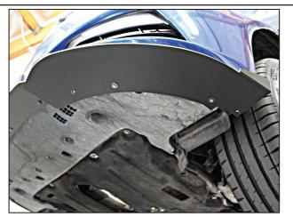
Attach the front splitter-side pieces, first, using the factory screws in the factory holes. Loosely fasten screws for now.
