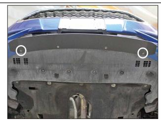
Reuse factory hardware for each mounting hole for the center splitter. Tighten hardware, but keep the two outside screws (circled above) loose until the end of installation.
