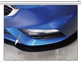
Line up the side pieces with the center section before marking the holes to drill in the next step.
