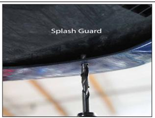
Follow through with a normal 5/16inch drill bit and make sure to drill through the splash guard located above the bumper.
