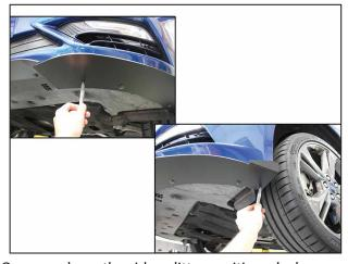
Once you have the side splitter positioned where you want it, mark the remaining holes for drilling.
