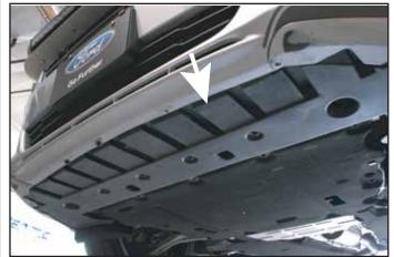
Use 7mm socket and Torx screwdriver to remove the front splash guard for easy access to fog lights. Splash guard is shown with white arrow.
