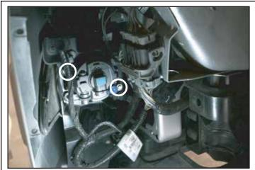
Disconnect the plug connected to the Fog Lights.
