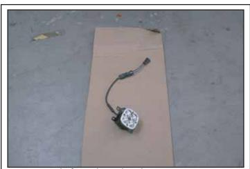
Optional: If purchased with H11-Baja Designs harness, attach the harness. Make sure the black wire connects to the receiving black wire on the LED Lights
