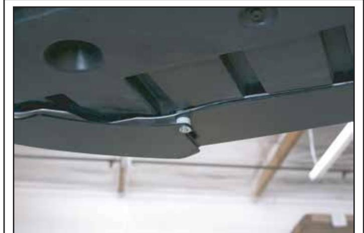
Slide the nylon spacer between the center and side pieces of the splitter. Attach the supplied #8 screw with the 1/4" washer.
