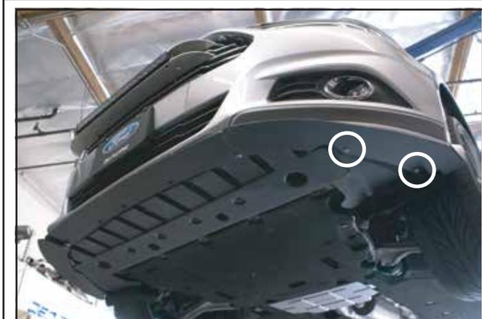
Install the side pieces using the 1/4" hardware. Only attach the hardware circled in white.
