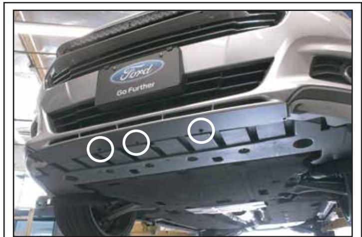
Attach the middle splitter to the car. Use the factory hardware for 3 middle holes as circled. **Note:** Do not screw in the holes on the side.
