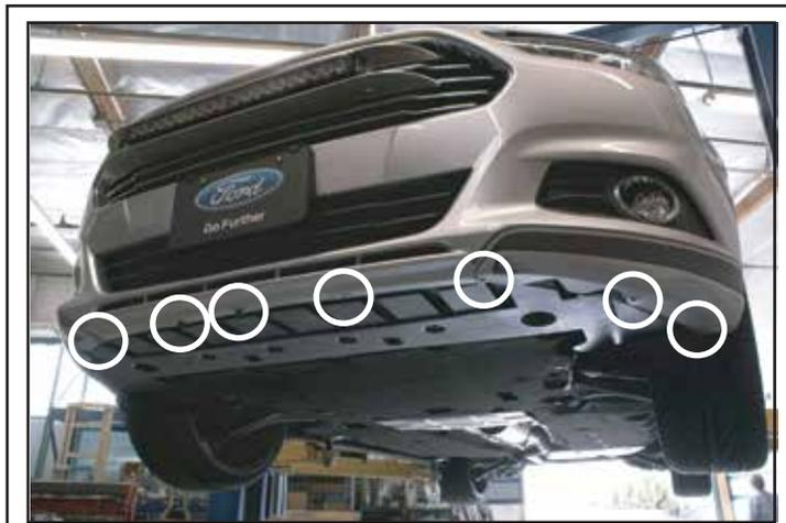
Remove (9) #8 screws from the front of the bumper. They are circled in white, respectively.
