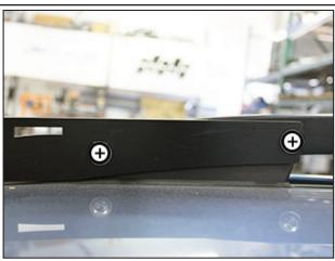
Using the mount holes as a template, mark the center holes for drilling on the roof rail. Start with a small bit to create a pilot hole, then drill out the holes to 25/64".
