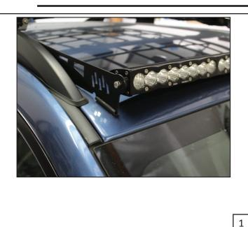
Set the left mount on the inside of the factory roof rail like so. The edge of the mount should sit flush with the opening on the roof rail.
