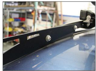
Fasten the left mount to the roof rail with (1) 1/4"-20 x1"
