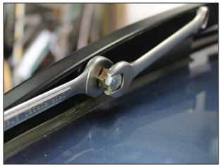
Using Riv Nut Tool Set: Tighten bolt clockwise using a 7/16" wrench while holding the collar steady, in place, with a 5/8" wrench.
