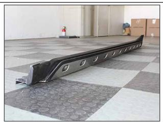
Set the factory rocker panel on top of the new rocker panel guard. Ensure it sits right up against the guard. Carefully turn over the assembly to mark the locations for the mounting holes on the bottom.
