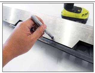
Mark the mounting holes for drilling on the rocker panel using the pre-drilled holes on the rocker panel guard as a template. Note: Only (6) holes need to be drilled to mount the new panel to the factory panel.
