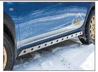
Reinstall the rocker panels in the factory location and return all factory fasteners to corresponding holes.
