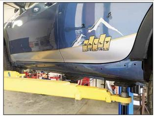
Remove the factory rocker panels. There are (5) large fasteners underneath and the front mudflaps that need to be removed. Be careful when prying the panel off the car to preserve the factory clips.
