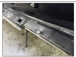
Drill out the (2) end holes with a 1/4" drill bit and install the 1/4" hardware in the orientation as follows, 1/4" Buttonhead Bolt (head facing the sky), 1/4" Washer, Spacer (inbetween the rocker guard and factory plastic), 1/4" Washer, and 1/4" Lock Nut. Repeat on the opposite end hole.
