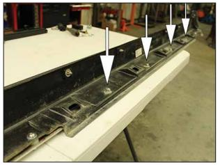
Drill out the (4) middle holes to 1/4". Install 1/4" hardware in the orientation as follows, 1/4"x3/4" Bolt & Washer (head facing the ground, insert up through rocker guard and factory plastic), 1/4" Washer, 1/4" Lock Washer, and 1/4" Nut. Repeat for each hole.
