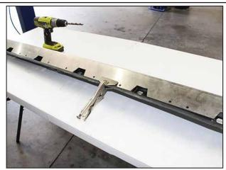
Helpful tip: Use a clamp to hold the two pieces in place while you mark the holes for drilling on the underside.
