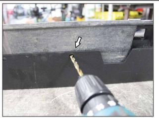
Helpful tip: Use a clamp to hold the two pieces in place while you drill the holes for mounting.
