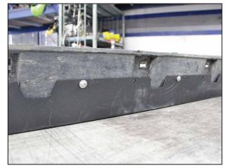
You can start installing the hardware as you move along drilling the mounting holes. Only (6) holes, spread out, across the entire rocker panel are needed. The orientation of the hardware is as follows: 1/4"-20 x3/4" bolt, 1/4" Washer, rocker panel guard, factory rocker panel, 1/4" Washer, 1/4" Lock Washer, and Nut.
