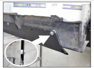
Install the longer 1/4"-20 x1" bolts into the front and rear-most holes in the orientation as follows: 1/4-20" Bolt, 1/4" Washer, rocker panel guard, 3/8" spacer, factory rocker panel, 1/4" Washer, 1/4" Lock Washer, and Nut.
