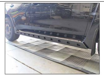
Reattach the rocker panels back to the vehicle.
