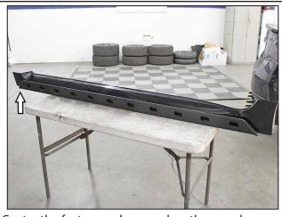
Center the factory rocker panel on the guard as much as possible. Our test vehicle measured roughly 2 - 1/8" away from the front edge.
