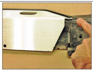
Align the front edge of the rocker panel guard to the factory panel as shown above.
