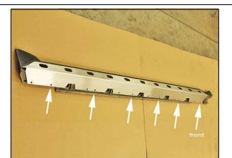
Only (6) holes are needed to mount the rocker panel guard to the factory plastic panel.
