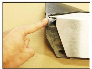
Align the rear edge of the rocker panel guard to the factory plastic as shown above.
