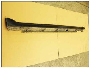
Remove the factory rocker panels. Note: There are (5) large fasteners, (1) Screw, and the front mudflaps that need to be removed. Be careful when prying the panel off the car to preserve the factory clips.
