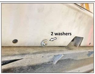
Install the shorter  $1/4''-20 \times 3/4''$  long bolts in the remaining (5) holes in the orientation as follows for each hole: 1/4''-20 bolt, (2) 1/4'' Washer, factory plastic guard, rocker panel guard, 1/4'' Washer, 1/4'' Lock Washer, and Nut. One side of rocker panel guard should now be completely fastened to the factory plastic panel. Repeat the previous steps on the opposite side.
