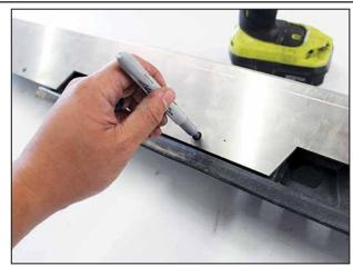
Mark the mounting holes for drilling on the factory plastic using the pre-drilled holes on the rocker panel guard as a template. Note: Only (6) holes need to be drilled in the plastic to mount the new panel to the factory panel.
