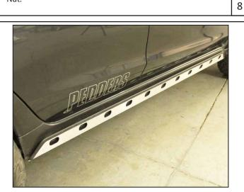
Reattach the rocker panels back to the vehicle.
