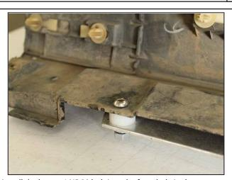
Install the longer 1/4"-20 bolt into the front hole in the orientation as follows: 1/4-20" Bolt, Spacer (inbetween rocker guard and factory plastic), 1/4" Washer, 1/4" Lock Washer, and Nut.
