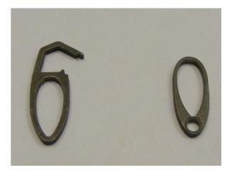
Both of the above fittings are designed To be tight, But they may require a little Cleaning /de burring on the inside edges to stop them Scratching off the anodising. But do not open out the fittings in size as This tight fit is all that stops them from Moving.
