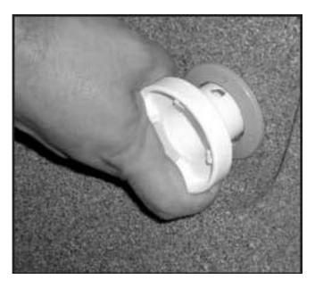
2. Insert the long part of the jet wrench and turn counter clock wise until there is no tension.
