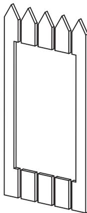
2. Slide the back box through the front of the fence. Screw it to the fence with the screws provided (for hardwood fences, it is easier to pre-drill the screw holes).
