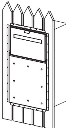
3. Attach the front panel by inserting the 8 x mounting studs through the corresponding holes in the back box. Reach through the back door and secure with the nuts provided.
