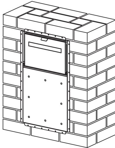
3. Once the brickwork and any rendering has been completed, attach the front panel by inserting the 8 x mounting studs through the corresponding holes in the back box. Reach through the back door and secure with the nuts provided.
