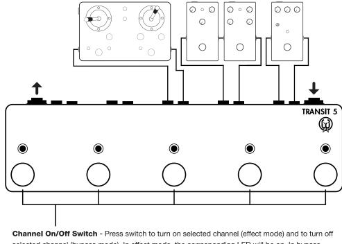
**Channel On/Off Switch** - Press switch to turn on selected channel (effect mode) and to turn of selected channel (bypass mode). In effect mode, the corresponding LED will be on. In bypass, the LED will be off.
