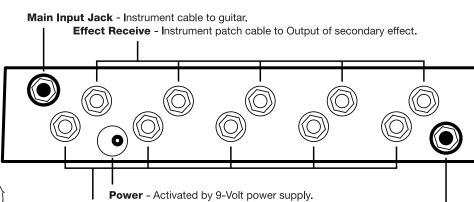
Effect Send - Instrument patch cable to Input of secondary effect.
