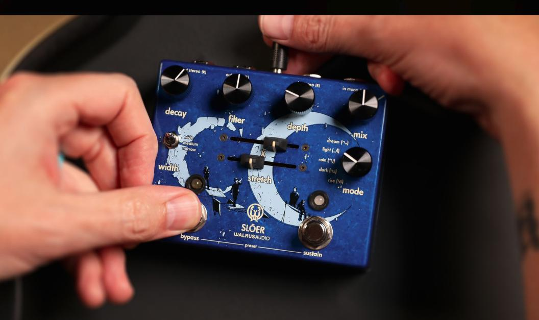
**Trails Mode:** The Slöer can run in trails or no trails mode. In trails mode, when you turn the pedal off, the reverb decay dies off naturally. In no trails mode, the decay is abruptly cut off when you turn the pedal off. To toggle between either mode, hold down the bypass switch for 1 second while applying power to the pedal. Unplug power and repeat to toggle to the other mode. Default is Trails mode.
