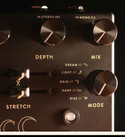
**Mix:** Control the amount of wet/dry mix. Fully left = dry. Fully right = wet.
