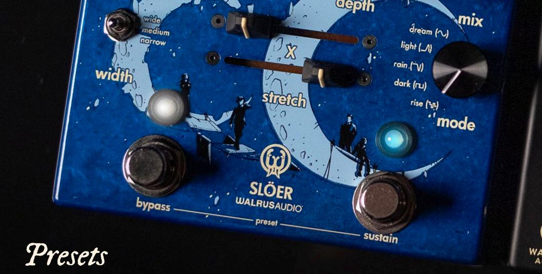
Slöer has three on-board presets (Red, Green, Blue). If the same algorithm is used in the next preset, the reverb sound spill over into the saved settings.
