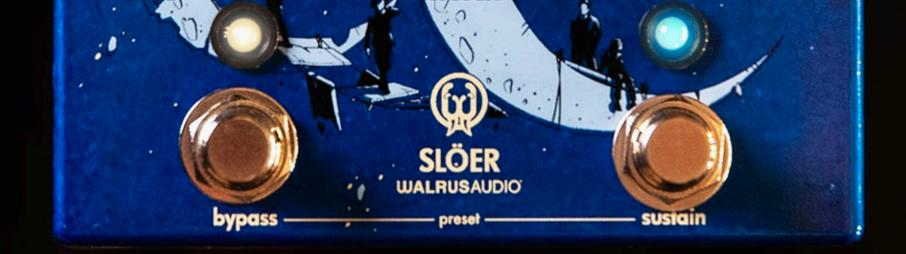
**Bypass Switch:** Turns the effect on and off. It also features our smart bypass switching. When the switch is in the off position, press and hold to temporarily activate the effect to add a moment of reverb texture. Releasing the switch turns the effect off, and fades it out.
