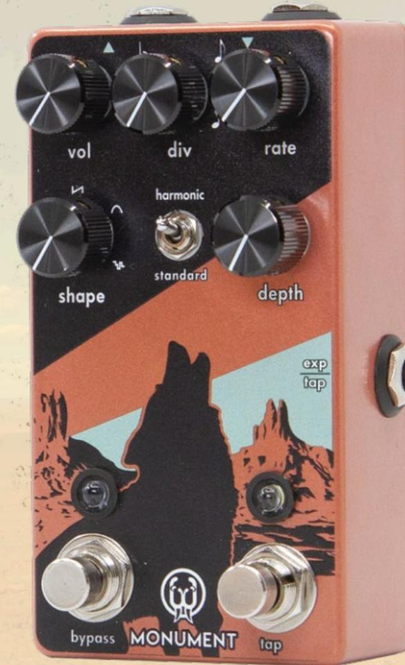
**EXPRESSION/TAP IN JACK** - Control parameters with a standard TRS expression pedal or set the time of the tremolo with an optional auxiliary tap switch.
